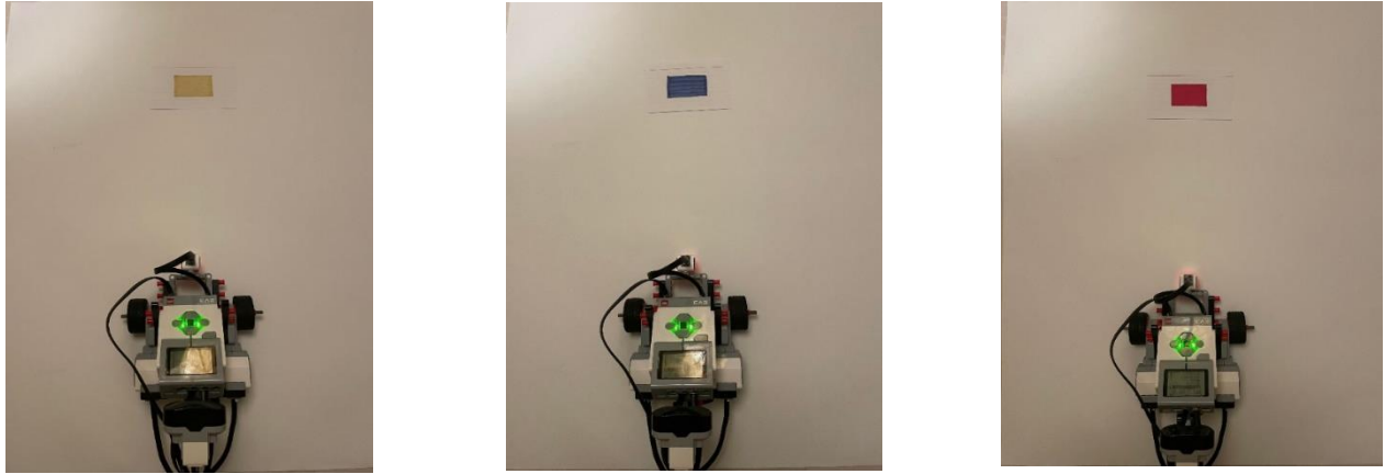
Figure 7: Color sensor trials with different colored index cards detected by robot.
