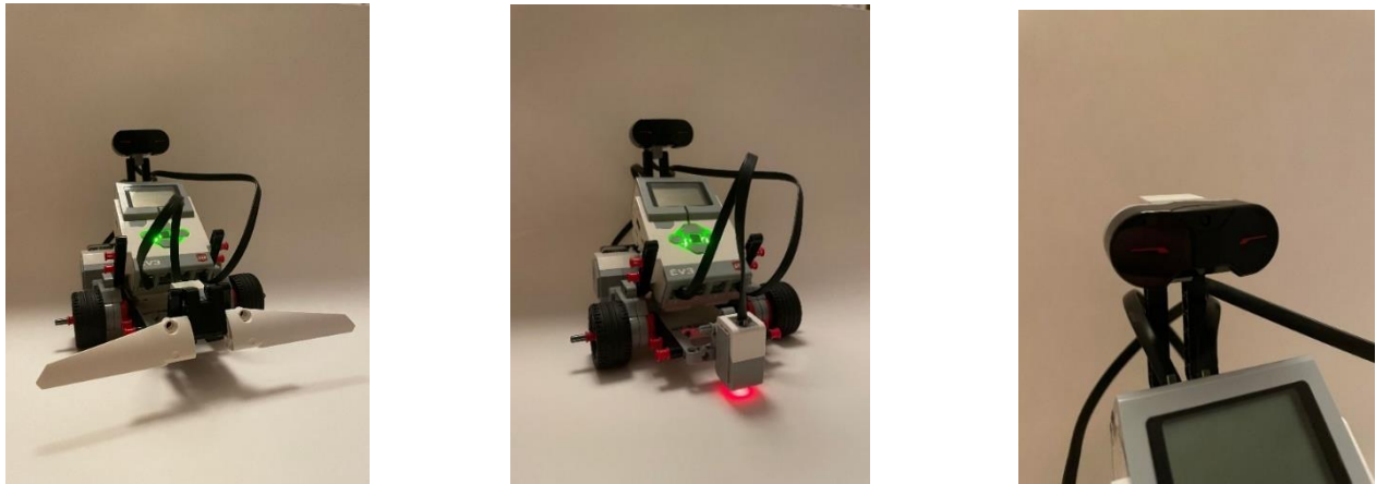
Figure 6: EXPLOR3R with (a) touch, (b) color, and (c) infrared sensors
