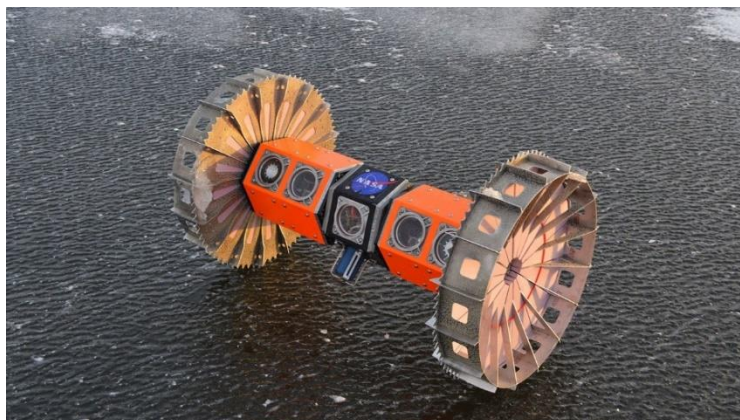
Figure 14: The BRUIE underwater exploration rover.
