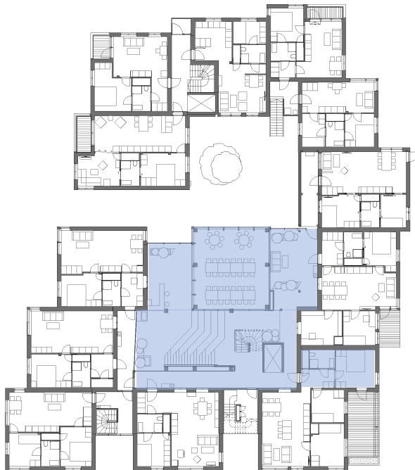
Fig. 8. Floor plan of Vindmøllebakken; common space in blue. (Illustration by Helen & Hard, Vindmøllebakken , Arkitektfirma Helen & Hard AS).
