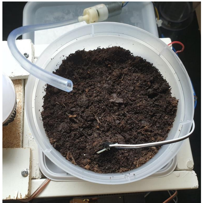
Figure 10: Image of the moisture sensor and water pump of the automated plant feeder
