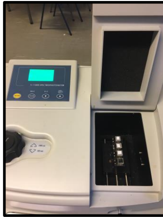
Figure 7. Measurement of the absorbance of the samples using V-1100 Spectrophotometer at 425nm
