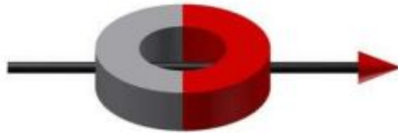
Figure 4: Magnetic field of an axially magnetised ring magnet (Magnetic Field)
