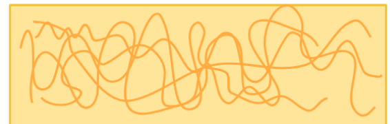
Tangled polymers in a unstretched rubber band
