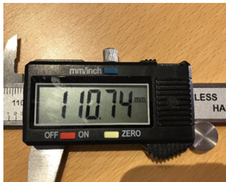
Figure 5: Digital calipers measuring 110.74mm \approx 11.0cm
