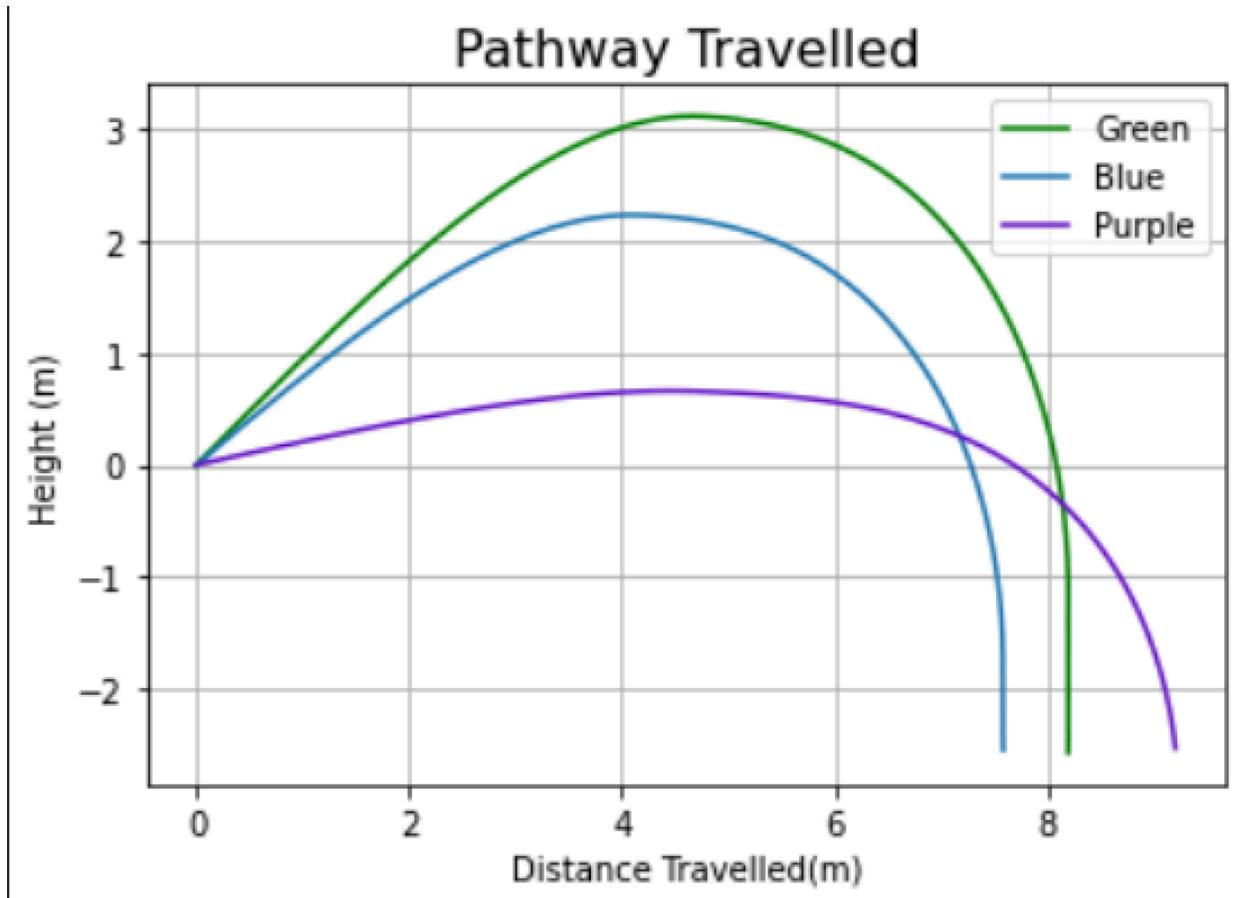
*Fig 18: My corresponding calculated trajectories to compare with three of Cohen's observed trajectories reproduced in Fig. 17.*
