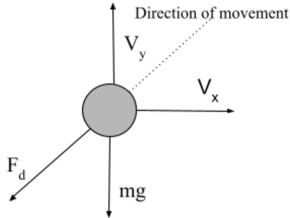
Figure 3: The dissociation of velocity of a badminton shuttle in air.
