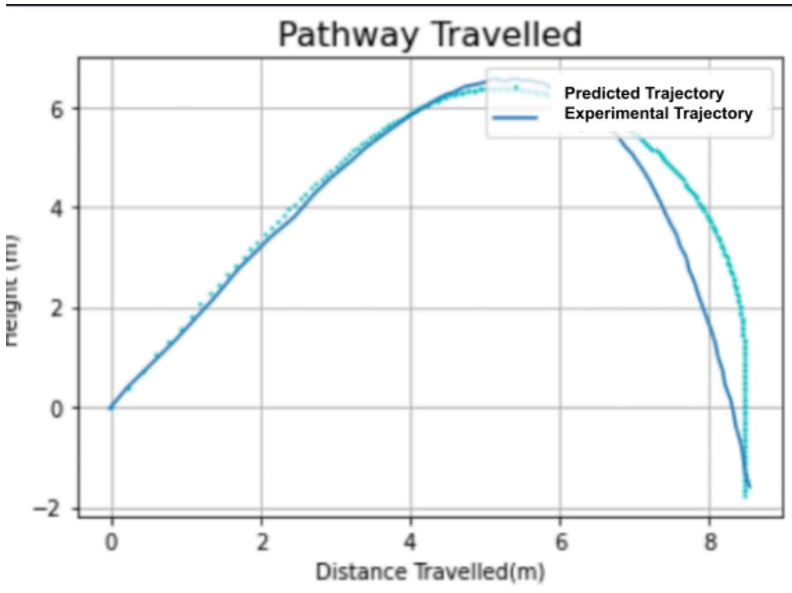
Figure 20: The Predicted Trajectory compared to the Experimental Trajectory in Python
