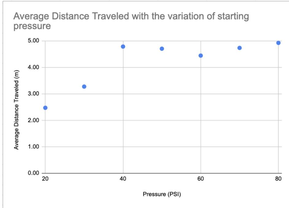
*Fig 16: Average distance measured behind the net a badminton clear shuttle landed with angle  $30^\circ$*
