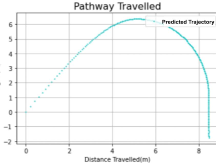
Figure 5: the predicted trajectory of badminton ball at  $V_0 = 44.3 \text{ m/s}$  and  $\Theta_0=60$
