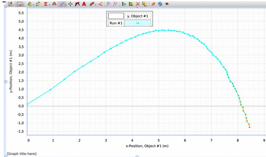
Figure 13: *Measured trajectory at  $v= 44 \text{ m/s}$ ,  $\theta= 20^\circ$*
